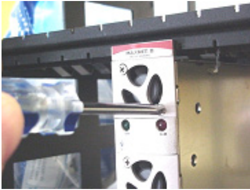
1. Remove two screws holding plate and fan in place.
