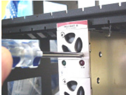
1. Remove two screws holding plate and fan in place.
